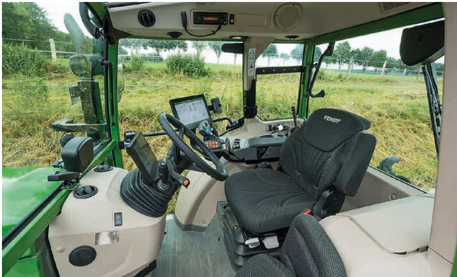
The new cab is quieter and gets the Fendt One operating set-up.
