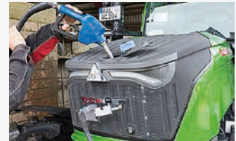
Don't spill it! The AdBlue filler is on the bonnet.
