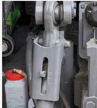
Each lift rod has a useful scale.
