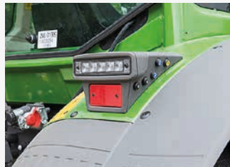
Linkage, a spool and the pto can all be operated from the ground.
