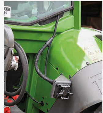
The ISO bus wiring is routed separately.
