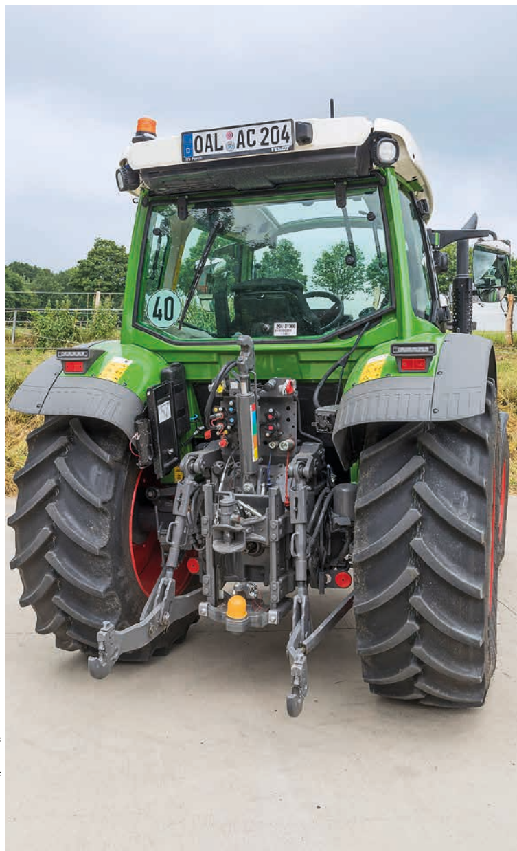
The back-end of the 211 Vario boasts plenty of hydraulic power, but it does lack some lift arm muscle.
