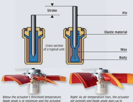
blade angle is at minimum and the actuator pin retracted.
