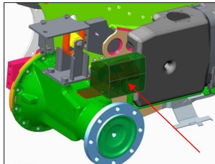
For installation at the rear axle, mounting bracket AL209191 must also be ordered from John Deere.
