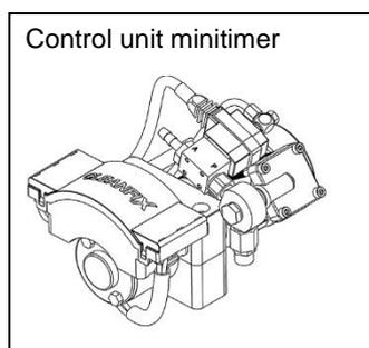
Briefly press the push button to automatically switch from cooling to cleaning and back again.
