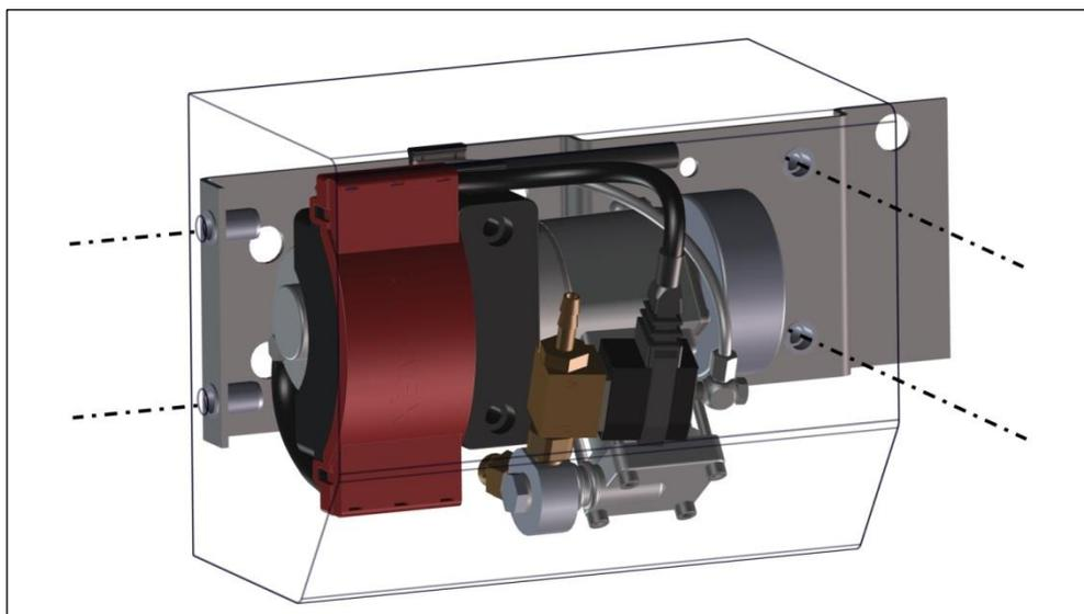
Remove the cover below the connector holder.
