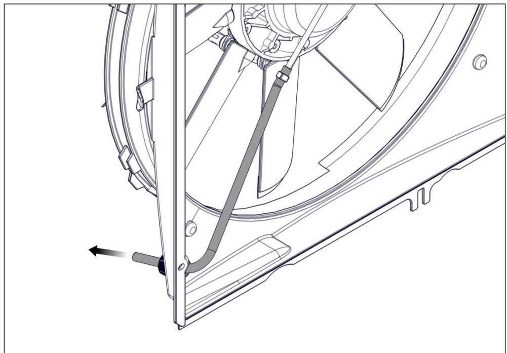
**NOTE****Property damage due to excessive tension on the pressure hose!**
