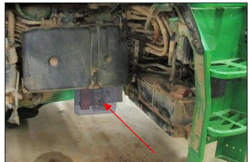
The attachment points provided for the compressed air system can be used for attachment.
