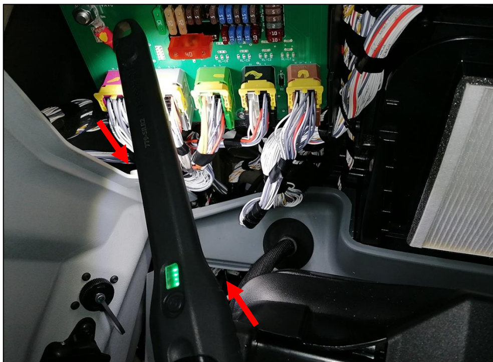
Plug for the cable gland: view from inside the cab in the back at the right
